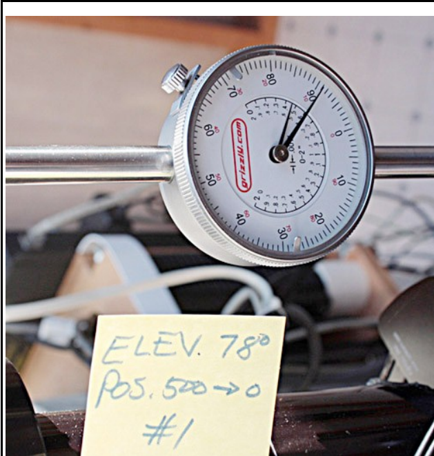
Illustration 6: Inward movement end position 0 returning from 500, 78°, motor speed 255. Reading is 91 thousandths, (0.009" too far) shown in table 2.
