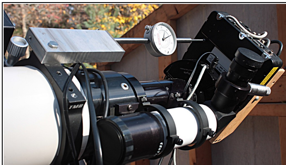
Illustration 1: Repeatability test setup.
