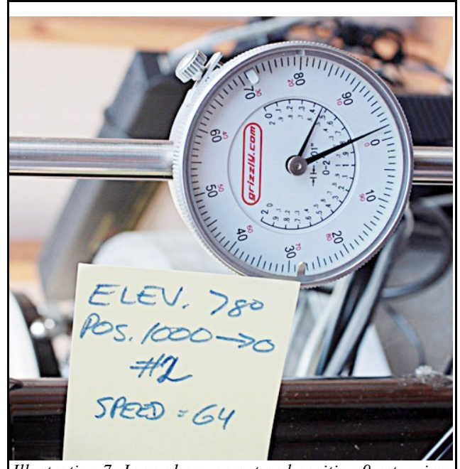
Illustration 7: Inward movement end position 0 returning from 1000, 78°, motor speed 64. Reading is 98 thousandths, (0.002" too far) shown in tables 4 and 5.
